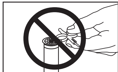
INCORRECT WAY TO ADJUST ARC
