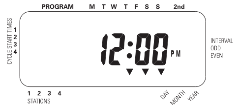
Figure 1: LCD Display with Surrounding Information
